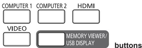
1) Press the <COMPUTER 1>, <COMPUTER 2>, <HDMI>, <VIDEO> or <MEMORY VIEWER/USB DISPLAY> button on the remote control.
