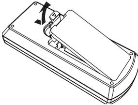
2. Remove the batteries.
