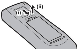
**2. Remove the batteries.**
