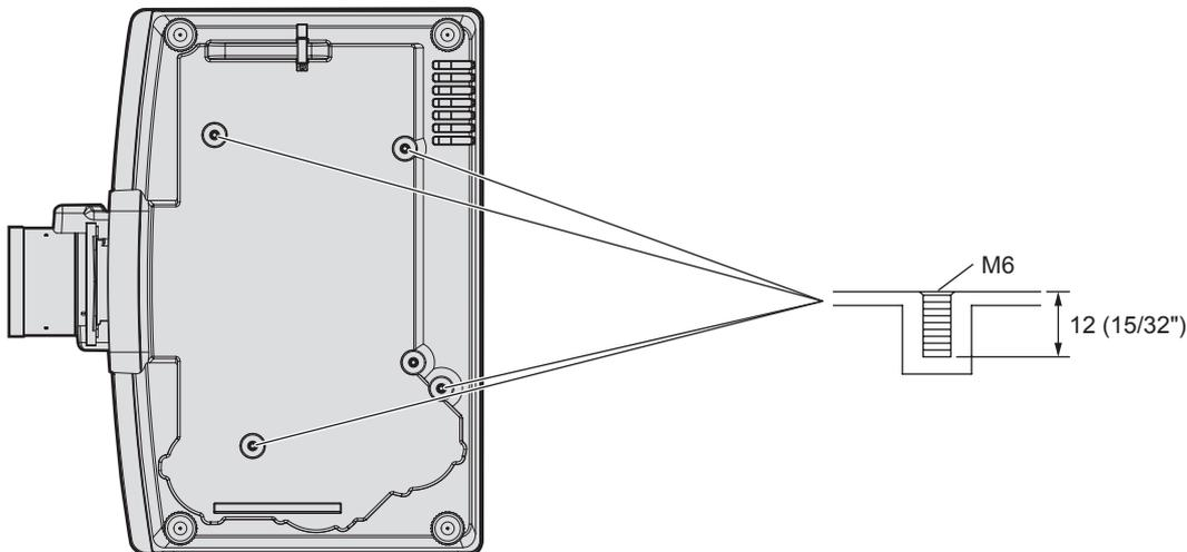
■ Dimensions for the screw holes to fix the projector (projector bottom view)
