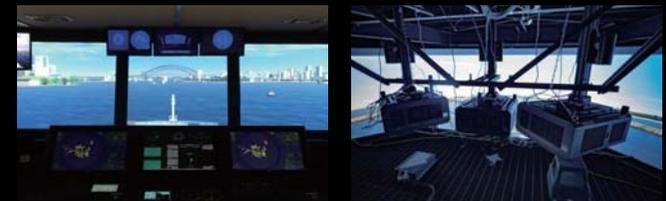
A total of five PT-RQ13K projectors were installed for seamless panoramic display.
