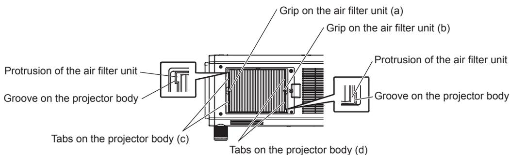
**1) Attach the air filter unit to the projector.**
