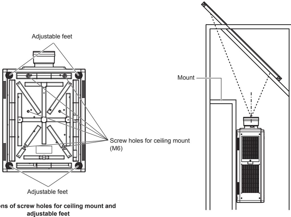
Positions of screw holes for ceiling mount and adjustable feet
