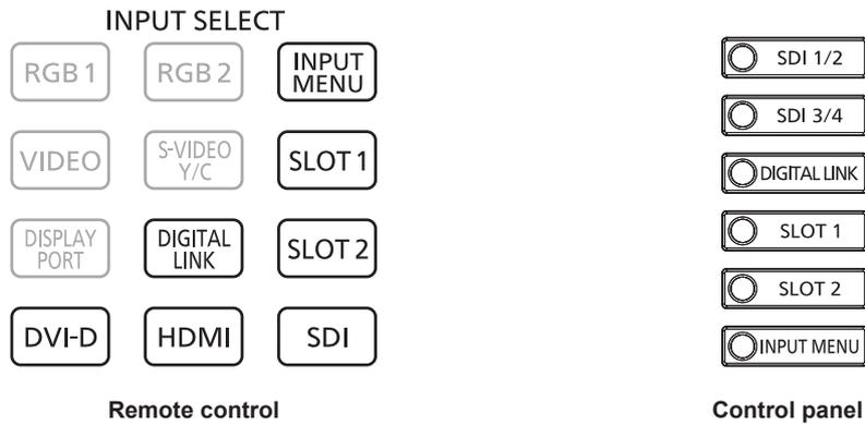
The input for projection can be switched. Method to switch the input is as follows.
