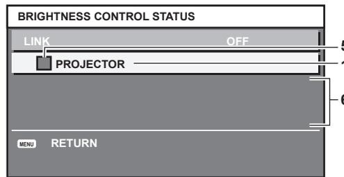
When [CONSTANT MODE] of [BRIGHTNESS CONTROL SETUP] is set to [AUTO] and [LINK] is set from [GROUP A] to [GROUP D]
