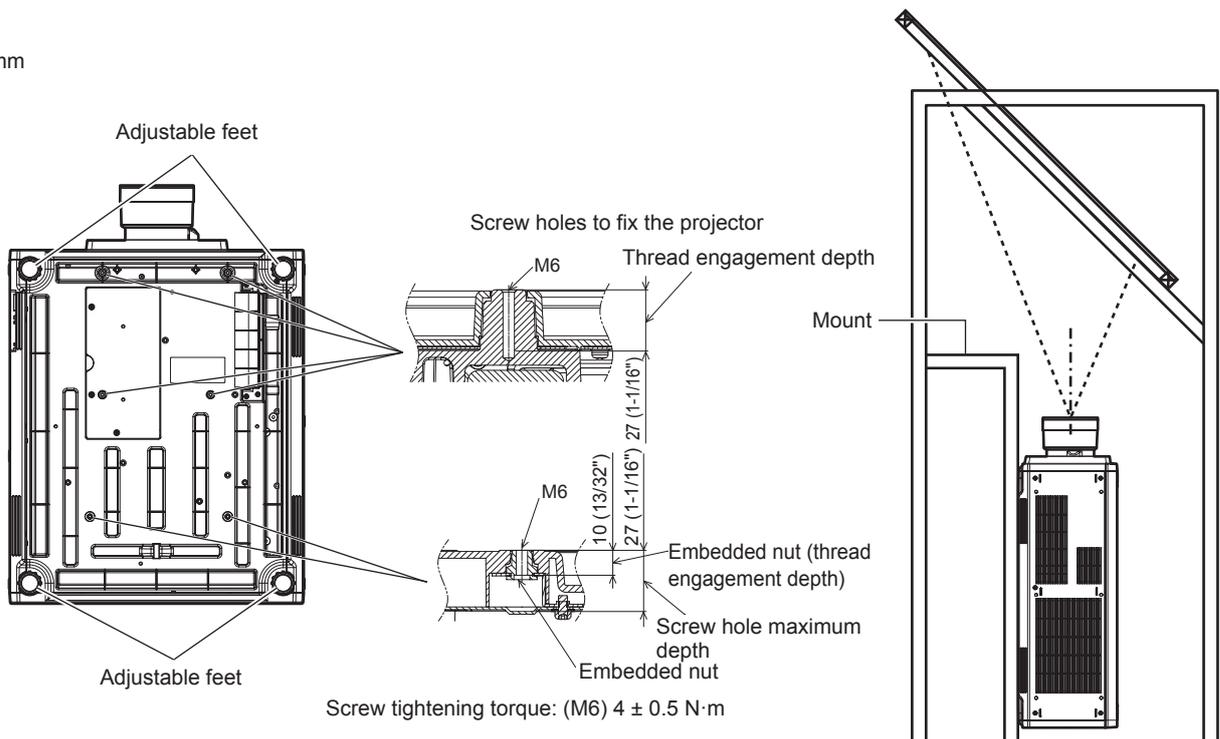
Screw tightening torque: (M6)  $4 \pm 0.5$  N·m
