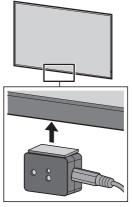
4 Connect the other terminal of the 4-pole micro plug cable to the SENSOR IN terminal.
