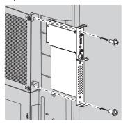
Tightening torque guideline: 0.5 N⋅m or less
