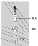
2 Attach the eyebolt and nut on the mounting position (two locations).
