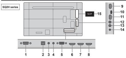
1 SERIAL IN: SERIAL Input Terminal
