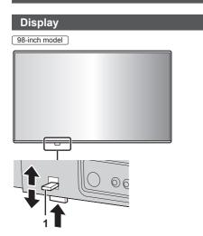
Slide the lever on the rear panel to eject the power indicator and remote control sensor.
