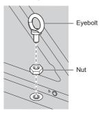
3 After removing the eyebolt, attach the bolt and nut.
