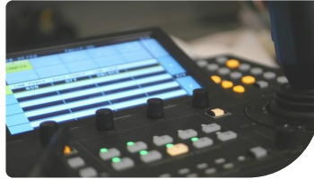
The Panasonic RP150 controls up to ten cameras simultaneously
