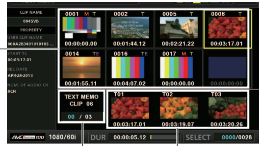
Thumbnail display Blue indicates selected number of text memo clips and white indicates total number of text memo clips. Indicates still images included with the text memos.
