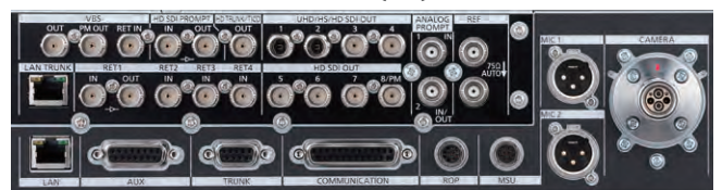
Rear of AK-UCU600 camera control unit (CCU)
