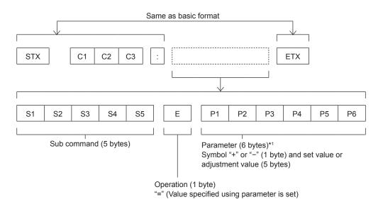
\*1 When transmitting a command which does not need a parameter, the operation (E) and parameter are not necessary.
