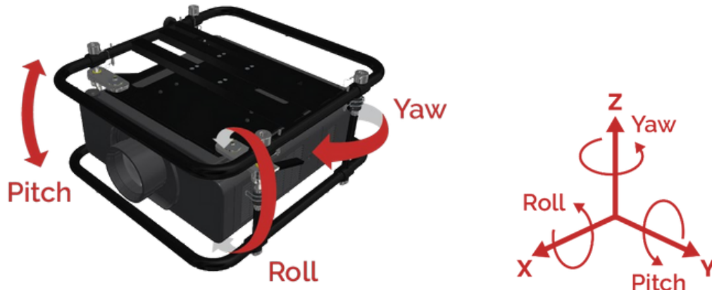
Figure 16 Illustration of yaw, pitch and roll
