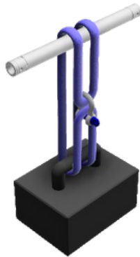
Figure 22 Illustration of basket hitch with a double wrapped rigging sling
