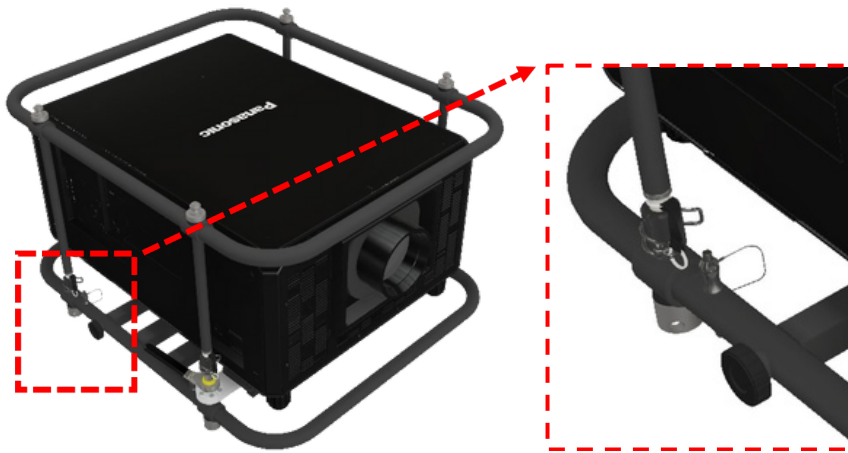
Figure 30 Locking pins at the frame
