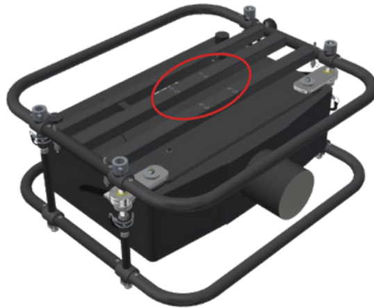
Figure 19 Threaded holes on bottom side of frame
