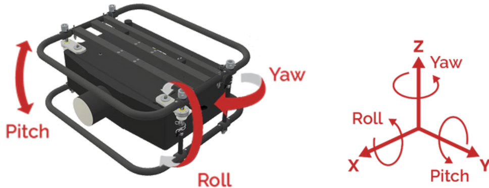
Figure 14 Illustration of yaw, pitch and roll
