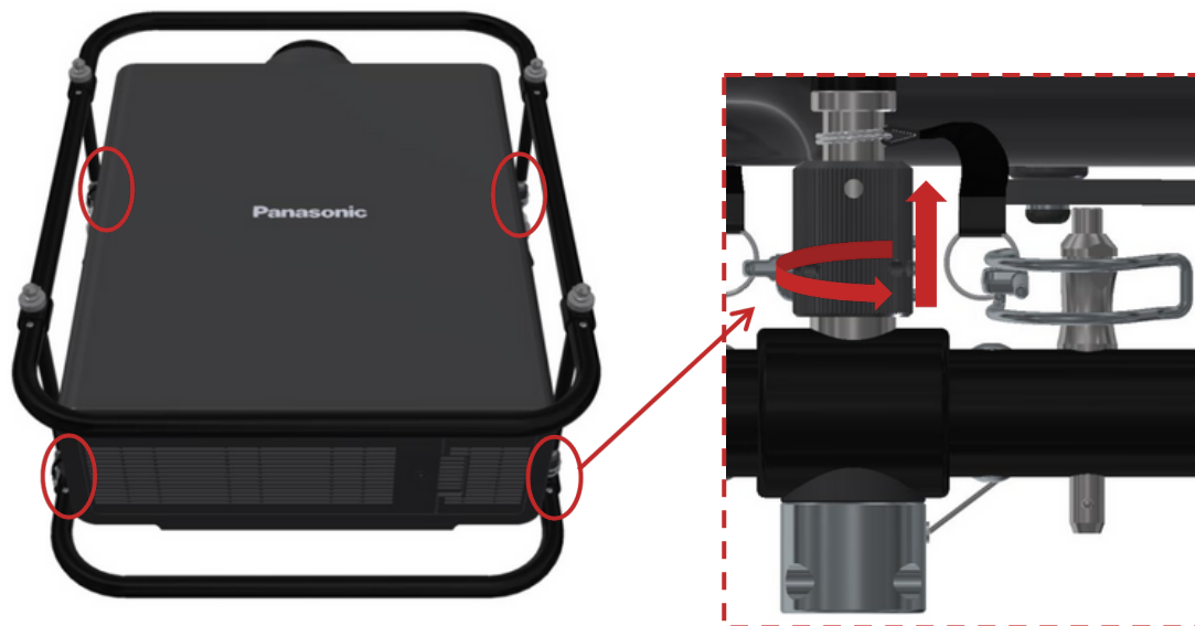
Figure 9 Unscrew the four attachment nuts
