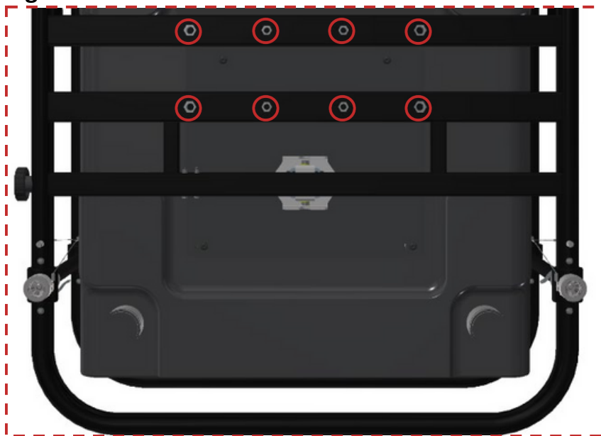
Figure 25 Inspection of mounting threads at bottom side
