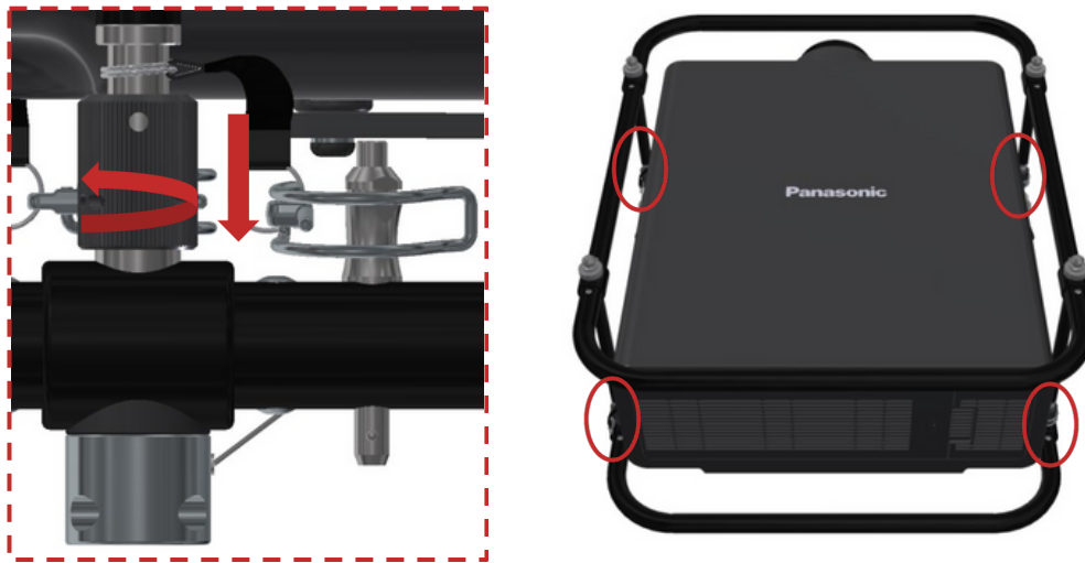
Figure 14 Tighten the four attachment nuts
