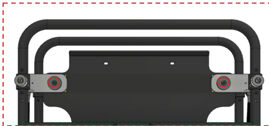
Figure 26 Nuts on front bottom side which are sealed with red colour wax
