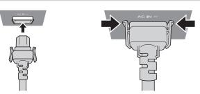
1) Check the shapes of the <AC IN> terminal on the side of the projector and the power cord connector, and insert the connector completely in the correct direction (until you hear the side tabs click in place).
