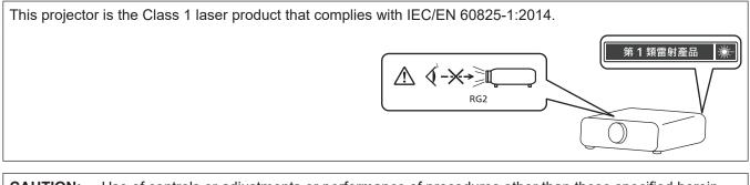
**CAUTION:** Use of controls or adjustments or performance of procedures other than those specified herein may result in hazardous radiation exposure.
