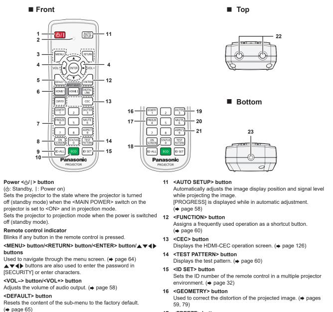
Input selection buttons (<HDMI 1>, <HDMI 2>, <DIGITAL LINK>, <COMPUTER>)
