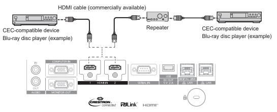
Connection example with CEC-compatible device
