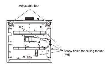
Positions of screw holes for ceiling mount and adjustable feet
