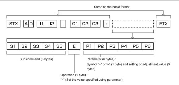
\*1 When transmitting a command which does not need a parameter, an operation (E) and parameter are not necessary.
