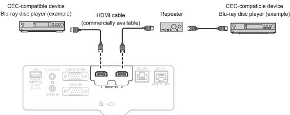
Connection example with CEC-compatible device
