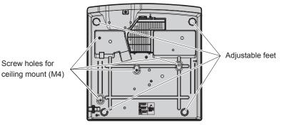
Positions of screw holes for ceiling mount and adjustable feet
