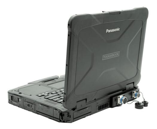
Equipped with a fully rugged design, a specialised module and a shock-proof mount, the TOUGHBOOK 40 Tactical delivers superior in-vehicle connectivity for wheeled and tracked military vehicles.
