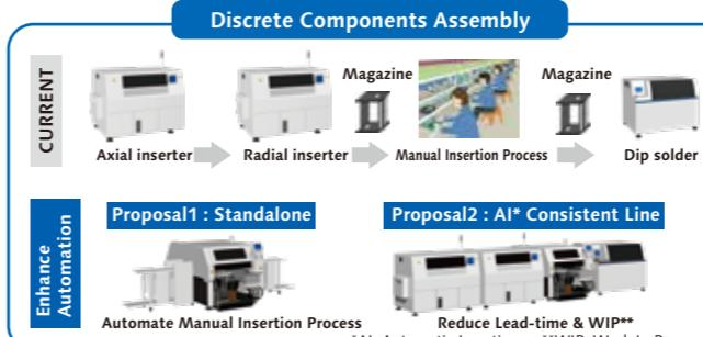
Convert manual insertion process to SMT inline process
