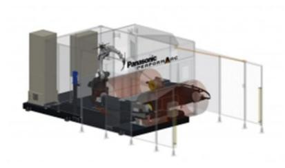
The Panasonic arc welding robot cell PERFORMARC FW-3PD (with 3 external axes PanaDice) is of a modular concept, developed using standard reliable Panasonic components.
